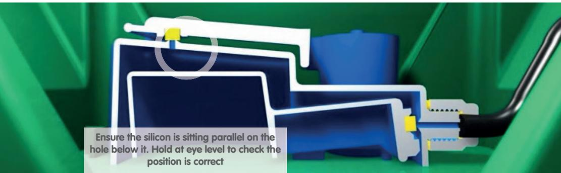
Ensure the silicon is sitting parallel on the hole below it. Hold at eye level to check the position is correct
